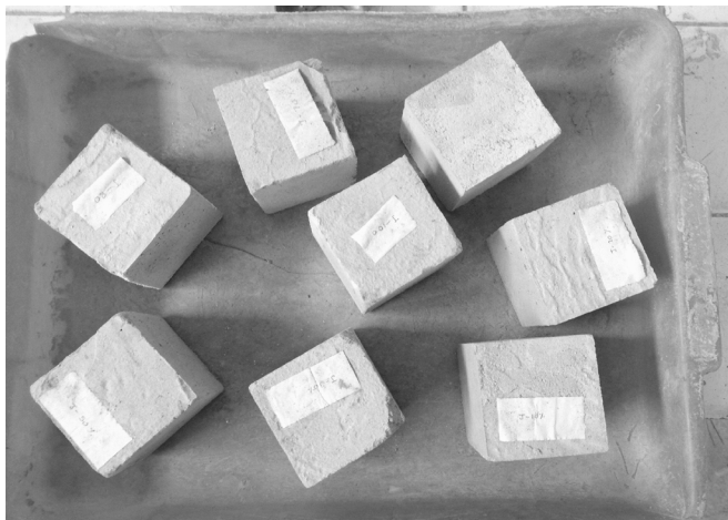
Fig. 7. Mortar cube specimens. Source: own study
