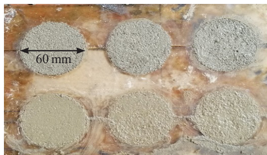
Fig. 4. Specimens to check thermal conductivity. Source: own study
