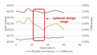
Figure 4. Glycol ratio effect on the solar fraction
