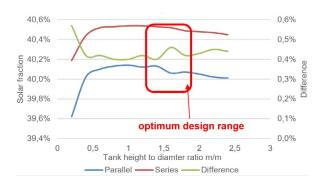
Figure 7. Tank height-to-diameter ratio effect on the solar fraction
