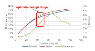
Figure 3. Collector area versus solar fraction
