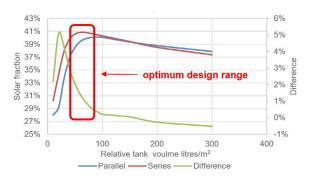
Figure 6. Relative tank volume effect on the solar fraction
