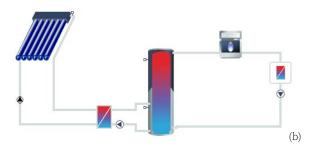
Figure 1. Solar thermal system for heat process (a) parallel boiler connection (b) series connection
